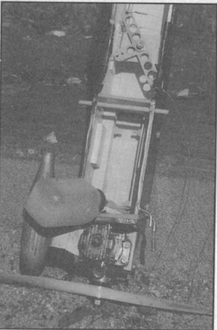
Easy access for attention to the fuel tank and bellcrank. Not everyone would take lightening the bellcrank so seriously...
